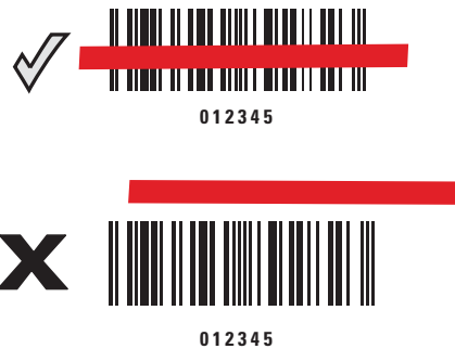
Figure 2-3 Scanning Orientation with Aiming Line
